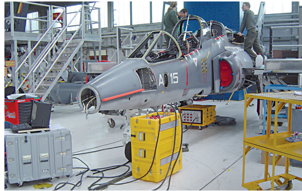
Used for aircraft MRO, ATE systems provide improved traceability, fault location and rapid aircraft turnaround.
